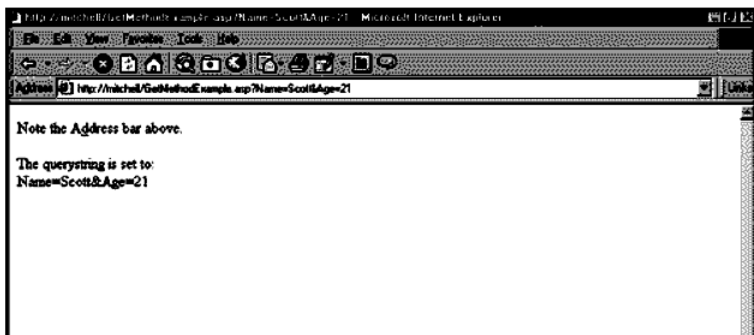
Figure 11.3. The form field values are stored as name/value pairs in the querystring.
