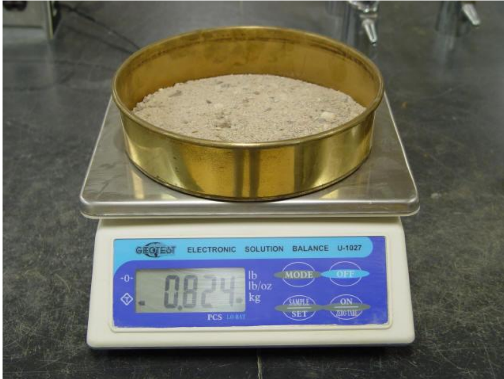
Fig: Illustrates Sieve Analysis test procedure
