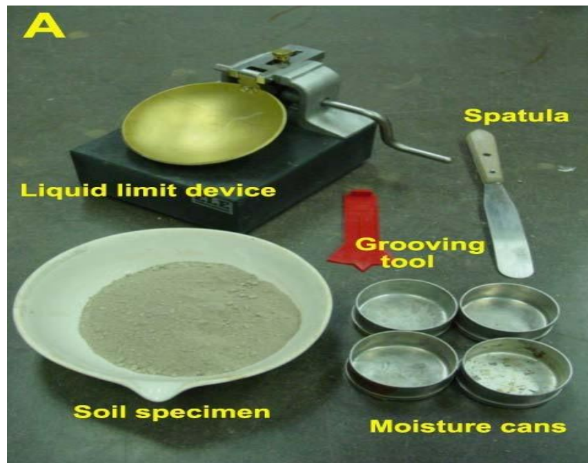
Fig: Shows Liquid limit test apparatus
