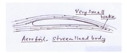
Fig. Flow over Bodies – Pressure Drag and Skin Friction Drag
