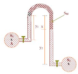
Inverted U-tube manometer is used to measure small difference in pressure between any two points. It consists of an inverted U-tube connecting the two points between which the pressure difference is required. In between there will be a lighter manometric liquid. Pressure difference between the two points can be calculated by writing the gauge equations for the system.
