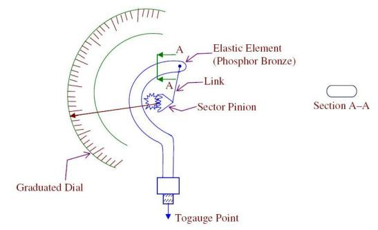
Mechanical gauge consists of an elastic element which deflects under the action of applied pressure and this deflection will move a pointer on a graduated dial leading to the measurement of pressure. Most popular pressure gauge used is Bordon pressure gauge.
