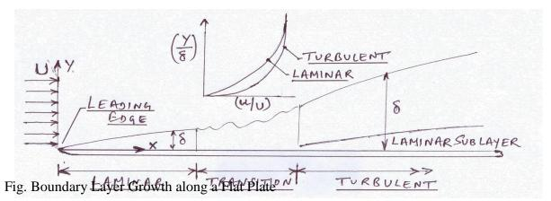
Up to a certain length along the plate from the leading edge, boundary layer thickness increases and the boundary layer exhibits the characteristics of a laminar flow irrespective of whether the incoming flow is laminar or turbulent. – This is known as laminar boundary layer. The thickness of the laminar boundary layer ( $\Box$ ) is given by ( $\Box$ ) = y (at (u/U) = 0.99)
