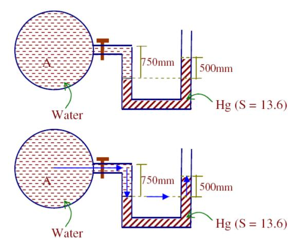
Let ' $h_A$ ' be the pressure head at 'A' in 'meters of water'.
