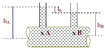
The arrangement consists of two pizometers at the two points between which the pressure difference is required. The liquid will rise in both the piezometers. The difference in elevation of liquid levels can be recorded and the pressure difference can be calculated.
