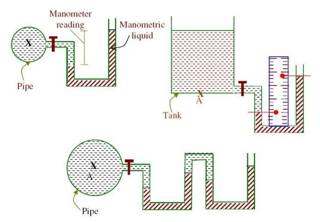
A U-tube manometers consists of a glass tube bent in U-Shape, one end of which
