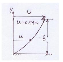
If the plate is smooth, the turbulent boundary layer consists of a thin layer adjacent to the boundary in which the flow is laminar. This thin layer is known as the laminar sub-layer.
