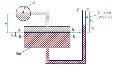
A single column manometer consists of a shallow reservoir having large cross sectional area when compared to cross sectional area of U – tube connected to it. For any change in pressure, change in the level of manometric liquid in the reservoir is small and change in level of manometric liquid in the U- tube is large.
