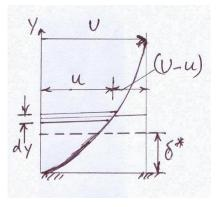
Fig. Displacement Thickness
