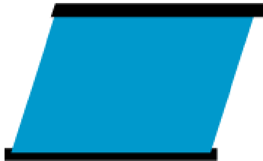
Fig.L-1.1a: Deformation of solid under a constant shear force
