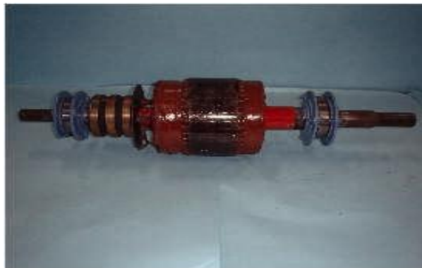
Figure 11: A wound rotor with slip rings
