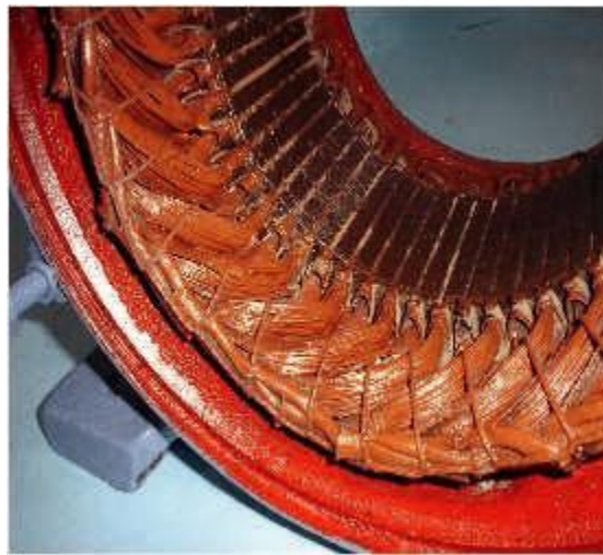
Figure 10: Coils in the stator
