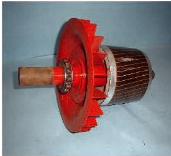
Figure 15: squirrel cage rotor
