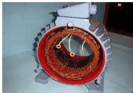
Figure 9: stator of an induction machine
