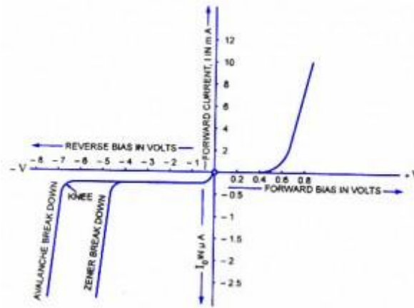
Fig 1.18: Diode characteristics with breakdown
