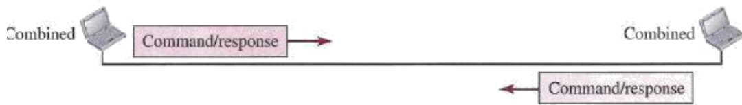
Figure 11.15 Asynchronous balanced mode
