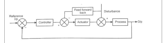
• In feedback system the disturbance must show up in the error before controller can take corrective action.
