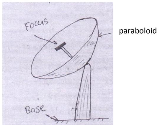
Working: A Paraboloida / dish collector brings solar radiation to a focus at a point actually a small central vol.
