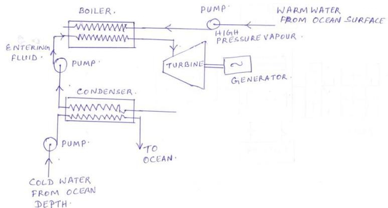
**Operation:** Warm water from ocean surface is circulated through a pump to a heat exchanger which acts as a boiler to generate working fluid ammonia vapour at high pressure.
