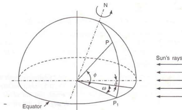
Figure 3.5 Latitude  $\phi$ , hour angle  $\omega$  and sun's declination  $\delta$ .
