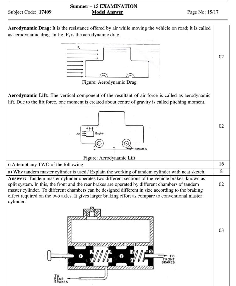
Figure: Tandem Master cylinder.
