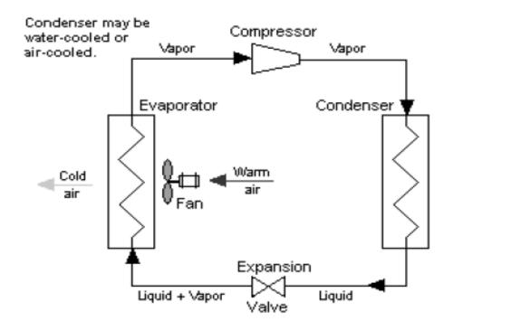
Figure: Layout of Vapour compression cycle.
