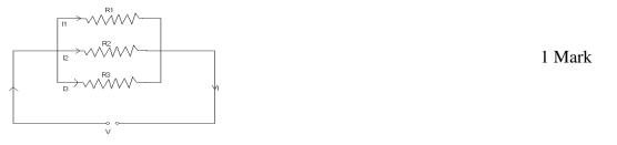
P.D. across all the resistances is identical and current in each resistor is different and is
