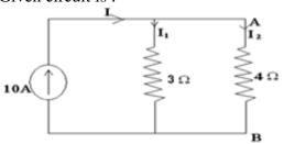
According to current division formula,<br/> $I_2 = [R_1 / (R_1 + R_2)] \times I$ 1 Mark<br/>1 Mark<br/>1 Mark<br/>1 Mark<br/>1 Mark<br/>1 Mark<br/>1 Mark $= [3 / (3+4)] \times 10$ <br/>= 4.285 A1 Mark<br/>1 Mark<br/>1 MarkTherefore, current through branch AB is 4.285 A.1 Mark<br/>1 MarkWhat are the thermal properties of good insulating materials?<br/>Ans:<br/>Thermal properties of insulating material:1
