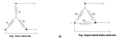
$$R_1 = (R_{12} * R_{31}) / (R_{12} + R_{23} + R_{31})$$
