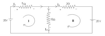
In loop I by KVL,  $20 - 5I_1 - 10I_3 = 0$  $\therefore 5I_1 + 10I_3 = 20$  ------(1)
