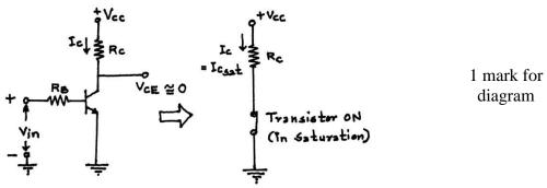
When  $V_{in}$  is positive, a large base current flows and transistor saturates. In the saturation region, both the junctions of transistor are forward biased. The collector current is very large, the voltage drop across the transistor ( $V_{CE}$ ) is very small, of the order of 0.2V to 1 V, depending on
