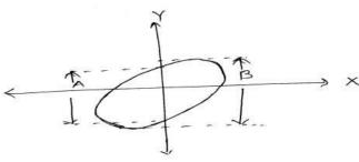
2. For phase difference above 900 and less than 1800, the ellipse appears. The phase shift is
