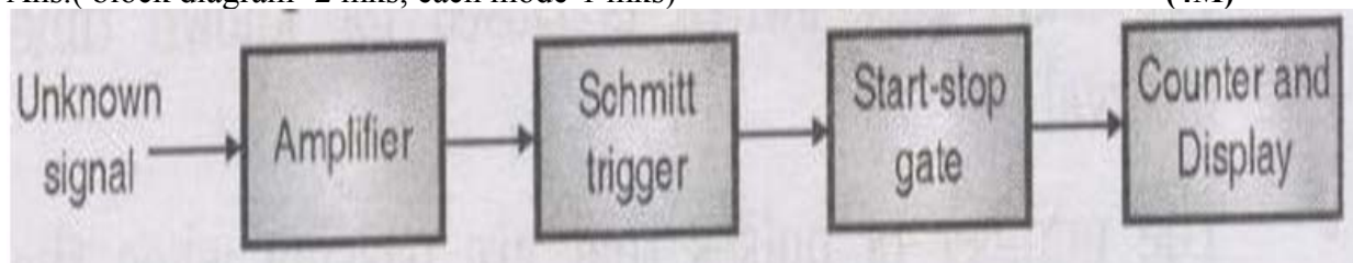
Fig. Block diagram of Digital Frequency Meter
