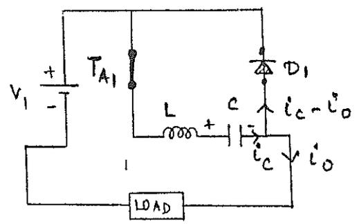
\* After SCR  $T_1$  is turned OFF, the capacitor current  $i_c$  increases further.
