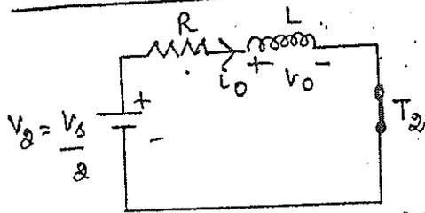
\* At  $t = t_3$ , when  $D_2$  is OFF, SCR  $T_2$  is turned ON
