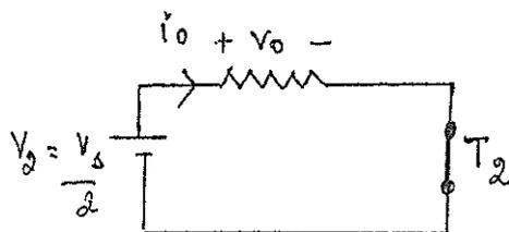
\*  $V_0 = -V_2 = -\frac{V_s}{2}$ ,  $i_0 = \frac{V_0}{R} = \frac{-V_s}{2R}$
