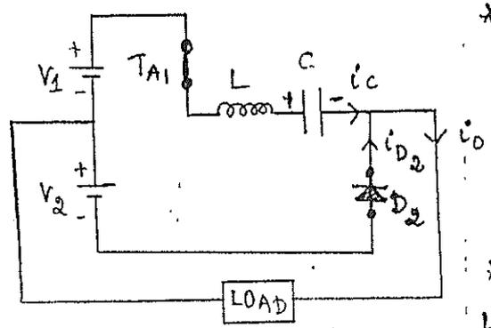
\* Now due to constant load current  $i_o$  the capacitor is slightly overcharged. i.e.  $V_c$  is slightly greater than  $V_s$  at  $t = t_4$ .
