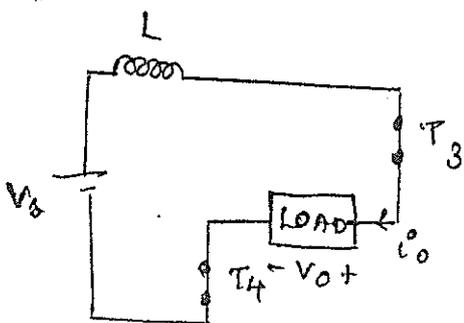
\*  $V_o, i_o$  is -ve when  $T_3, T_4$  is ON.
