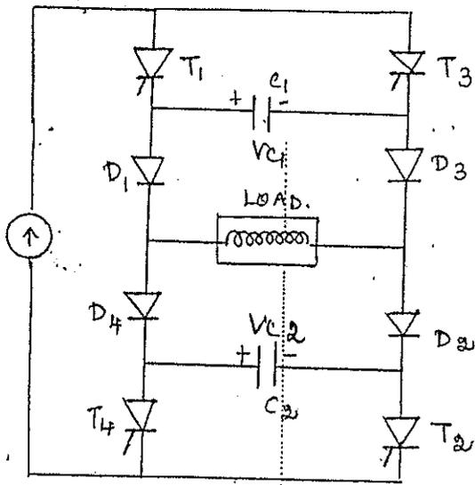
\* Capacitors are precharged with left plate +ve.
