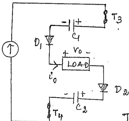
\* when  $T_3$  &  $T_4$  are ON, the capacitor voltage  $V_{C1}$  and  $V_{C2}$  apply a reverse bias across SCR  $T_1$  &  $T_2$  respectively and turns them OFF.
