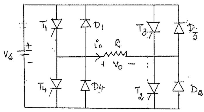
\* For R load, the diodes  $D_1, D_2, D_3, D_4$  does not conduct.
