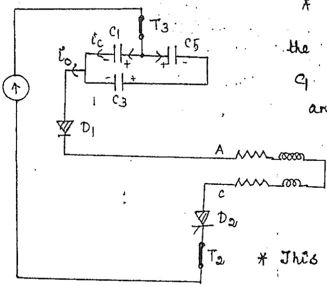
\* when  $T_3$  is turned ON, the voltage across the capacitor  $C_1$  reverse biases the SCR  $T_1$  and turns it OFF.
