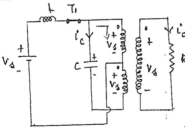
\* If say at  $t = t_3$  SCR  $T_1$  is triggered the capacitor voltage  $V_c = -2V_s$  reverse biases SCR  $T_2$  and turns it OFF.
