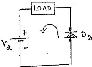
\* Now due to energy stored in load the diode  $D_2$  is forward biased.
