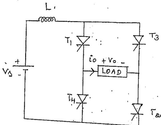
\* Inductor L in series with the  $V_d$  source, is to maintain the current constant.
