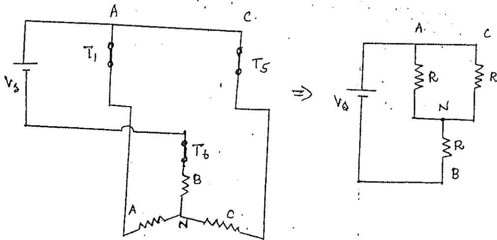
$R_{AN}$  and  $R_{CN}$  are in parallel.  $\therefore R_{eq} = \frac{R \times R}{R + R} = \frac{R^2}{2R} = \frac{R}{2}$
