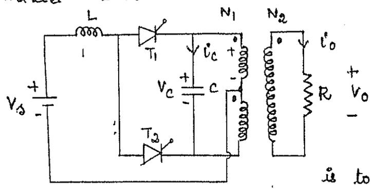
\* It uses two SCRs  $T_1, T_2$ .
