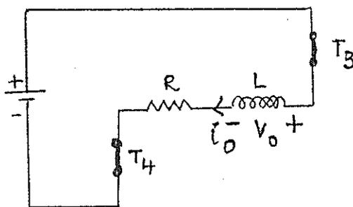
\* At  $t = t_3$ ,  $T_3$  and  $T_4$  are ON.
