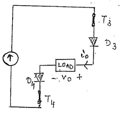
\* Now when  $D_1, D_2$  is OFF, the current  $i_o$  flows through  $T_3 \rightarrow D_3 \rightarrow \text{load} \rightarrow D_4 \rightarrow T_4$
