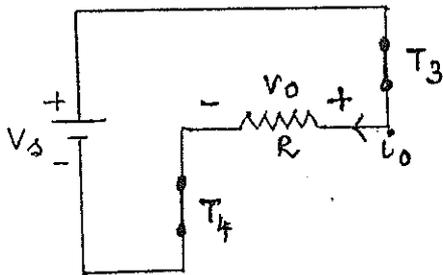
\* At  $t=T/2$ ;  $T_3, T_4$  are turned ON by giving gate pulses.
