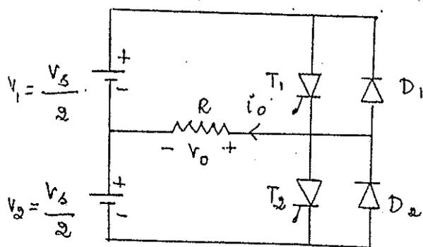
\* For R load D<sub>1</sub>, D<sub>2</sub> does not conduct.
