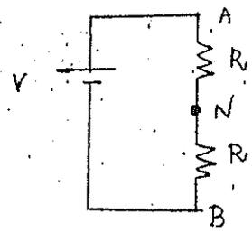
$V_{AN} = V_{BN} = V/2$
