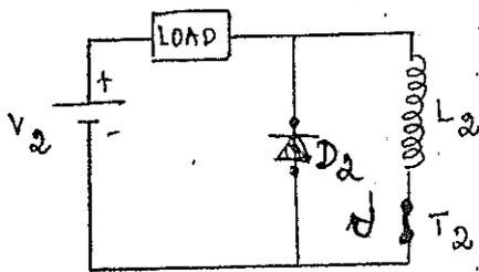
\* when capacitor is completely charged with lower plate +ve and upper plate -ve then diode  $D_2$  is forward biased.
