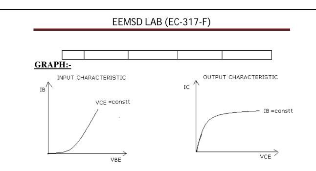
**<u>RESULT</u>**: The input and output characteristic of transistor in common emitter configuration has been plotted.
