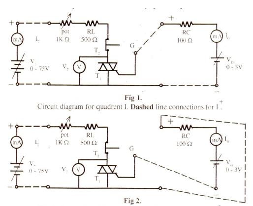
Circuit diagram for quadrent I. Dashed line connections for I.
