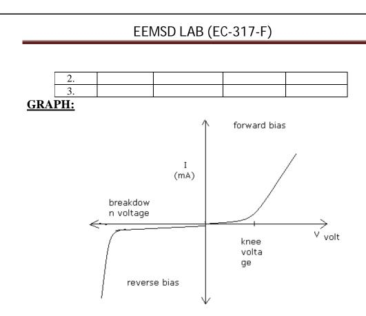
**<u>RESULT:</u>** The graph has been plotted between voltage and current.
