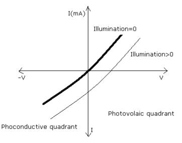
**<u>RESULT</u>**: The V-I characteristics of photo – voltaic cell has been plotted.
