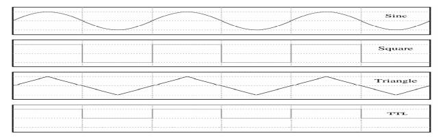
Fig:8 Waveforms of function generator
