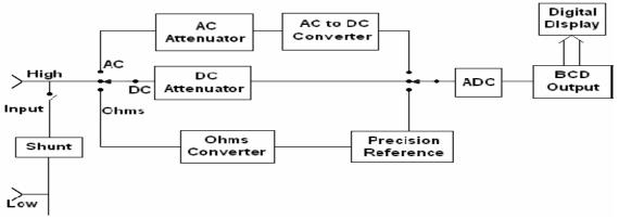
Fig:2 Block diagram of digital multimeter
