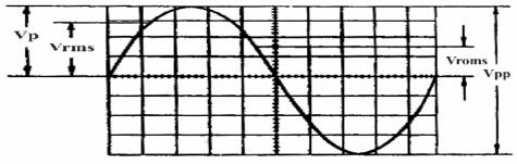
Fig:4 Amplitude measurement using CRO
