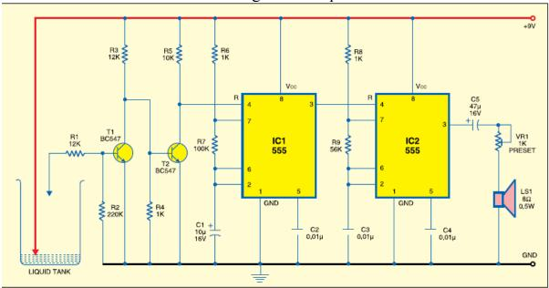
**PROCEDURE**: Assemble the circuit on a general purpose PCB and enclose in a suitable cabinet. Install two water-level probes using metal strips such that one touches the bottom of the tank and the other touches the maximum level of the water in the tank. Interconnect the sensor and the circuit using a flexible wire.
