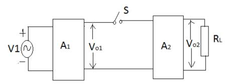
Two Stage amplifier (Block Diagram)
