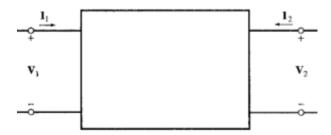
The parameters used in order to describe a two-port network are the following: Z, Y, A, h, g. They are usually expressed in matrix notation and they establish relations between the following parameters:
