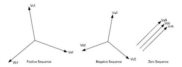
In all three systems of the symmetrical components, the subscripts denote the components in the different phases. The total voltage of any phase is then equal to the
