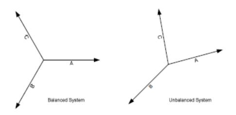
Consider the symmetrical system of phasors in Fig. 7.2. Being balanced, the phasors have equal amplitudes and are displaced 120 relative to each other. By the definition of symmetrical components,  $V \ b1$  always lags  $V \ a1$  by a fixed angle of 120 deg and always has the same magnitude as  $V \ a1$ . Similarly  $V \ c1$  leads  $V \ a1$  by 120 deg. It follows then that,
