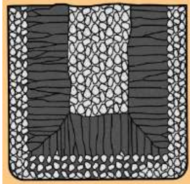
Figure 18 - Characteristic grain structure in an alloy casting, showing segregation of alloying components in center of casting
