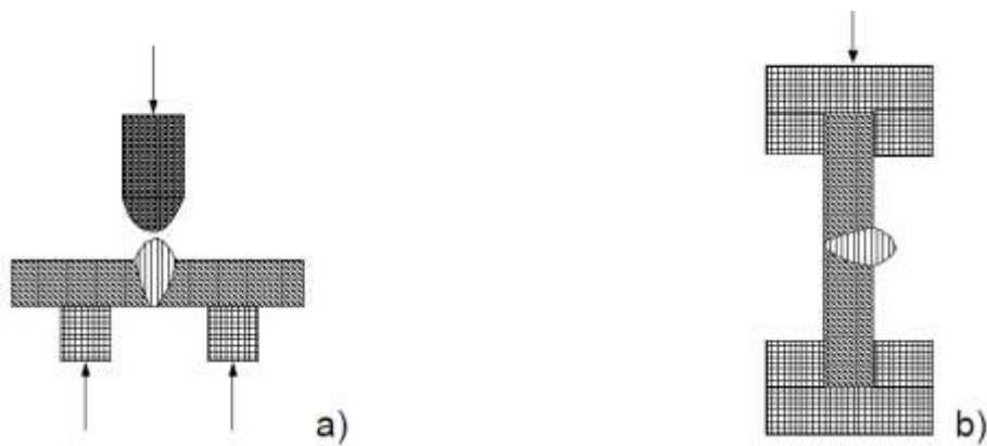
Fig. 84 Schematics of free bend tests
