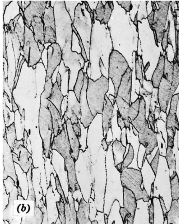
Anisotropic (directional) since rolling affects grain orientation and shape.
