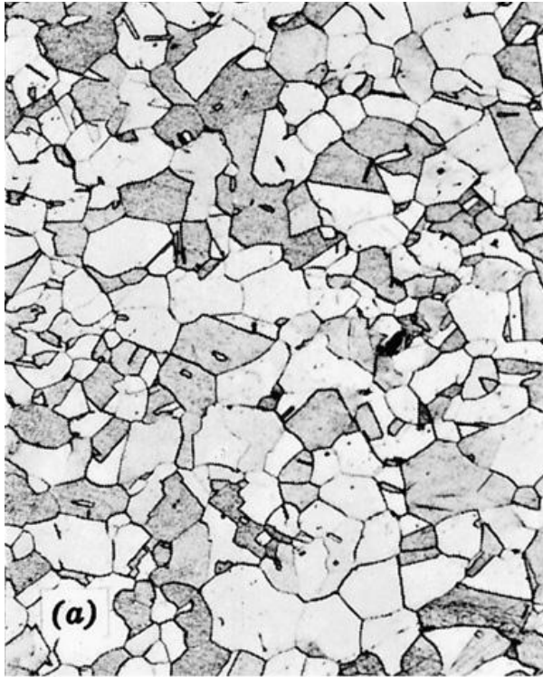
Isotropic grains are approx. spherical, equiaxed & randomly oriented.
