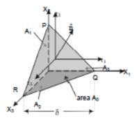
Figure 2: Consider an infinitesimal body at rest with a surface PQR that is not perpendicular to any of the Cartesian axis. The unit normal vector to that surface is  $\hat{n} = n_1\hat{x}_1 + n_2\hat{x}_2 + n_3\hat{x}_3$ . The area of the surface  $= A_0$ , and the area of each surface perpendicular to  $X_i$  is  $A_i = A_0n_i$ , for i = 1, 2, 3.
