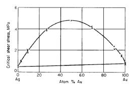
Figure Variation of critical resolved shear stress with composition in silver-gold-alloy single crystals.
