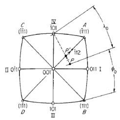
Figure Standard (001) stereographic projection or a cubic crystal.
