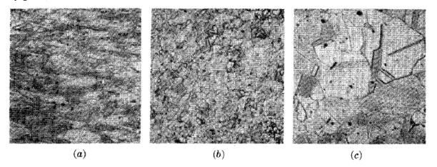
Figure 6-31 Changes in microstructure of cold-worked 70-30 brass with annealing, (a) Cold-worked 40 percent; (b) 440oC, 15 min; (c) 5750C, 15 min (150X)
