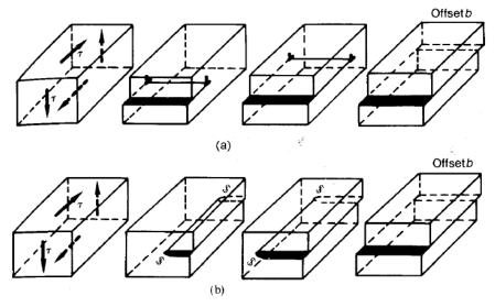
*Figure 5-4* (a) Macroscopic deformation of a cube produced by glide of an edge dislocation. (b) Macroscopic deformation of a cube produced by glide of a screw dislocation. Note that the end result is identical for both situations. '
