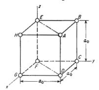
Figure 4-1 Simple cubic structure.
