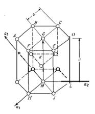
Basal plane (0001) ~ ABCOEF Prism plane (10TO) ~ FEJH Pyramidal planes Type I, Order 1 (10TI) - GHJ Type II, Order 2 (1012) - KJH Type II, Order 2 (1122) - KHL Digonal oxis [1120] - FGC
