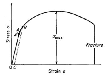
Figure 1-3 Typical tension stress-strain curve.
