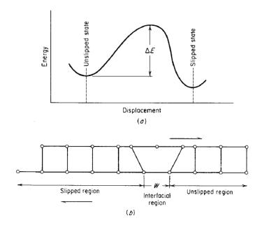
Figure (a) Energy change from unslipped to slipped state; (b) stages in growth of slipped region.
