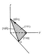
Slip direction in fee is <110> type direction. Slip directions are most easily established from a sketch of the (111) plane.
