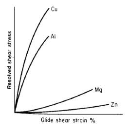
Figure Typical single-crystal stress-strain curves
