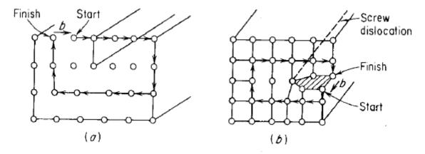
Figure 5-6 Burgers circuits, (a) Around positive edge dislocation; (b) around a right-handed dislocation.
