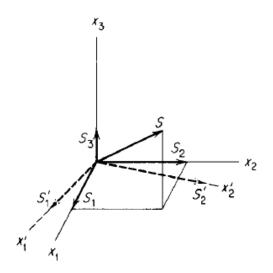
Figure 2-9 Transformation of axes for a vector
