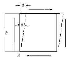
Figure 1-7 Shear strain.
