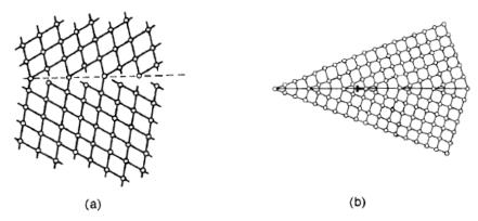
Figure 6-1 (a) Schematic atomic model of a grain boundary; (b) dislocation model of a rain boundary.
