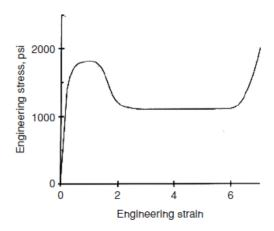
Figure Inhomogeneous yielding of a linear polymer
