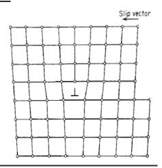
Figure Atomic arrangement in a plane normal to an edge dislocation
