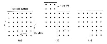
Figure 4-11 Schematic drawing of classical idea of slip.
