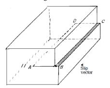
**Figure** Edge dislocation produced by slip in a simple cubic lattice. Dislocation lies along *AD*, perpendicular to slip direction. Slip has occurred over area *ABCD*.
