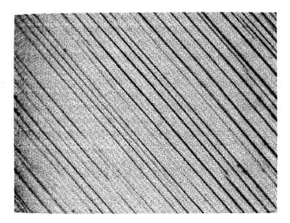
Figure 4-12 Straight slip lines in copper (500 × ). (Courtesy W. L. Phillips.)
