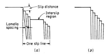
Figure Schematic drawing of the line structure of a slip band, (a) Small deformation; (b) large deformation
