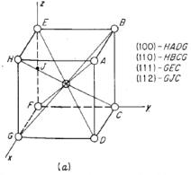
Figure 4-2 (a) Body-centered cubic structure
