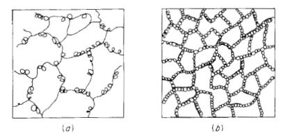
Figure 6-28 (a) Deformed to 10 percent strain. Beginning of cell formation with dislocation tangles; (b) deformed to 50 percent strain. Equilibrium cell size with heavy dislocation density in cell walls (schematic)
