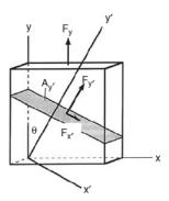
Figure 1.2. Stresses acting on an area, A', under a normal force,  $F_y$ . The normal stress  $\sigma_{y'y'} = F_{y'}/A_{y'} = F_y \cos\theta/(A_y/\cos\theta) = \sigma_{yy} \cos^2\theta$ . The shear stress  $\tau_{y'x'} = F_x/A_{y'} = F_y \sin\theta/(A_{yx}/\cos\theta) = \sigma_{yy} \cos\theta \sin\theta$ .
