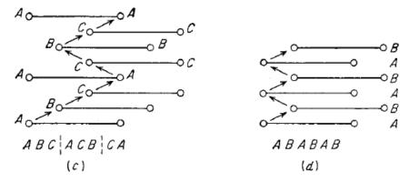
Figure Faulted structures, (a) fcc packing; (b) deformation fault in fee; (c) twin fault in fee; (d) hcp packing.
