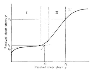
Figure 4-33 Generalized flow curve for fcc single crystals.
