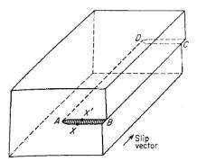
**Figure** Slip that produces a screw dislocation in a simple cubic lattice. Dislocation lies along AD, parallel to slip direction. Slip has occurred over the area ABCD.
