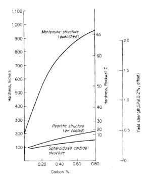
Figure 6-26 Hardness of various transformation products in steel.
