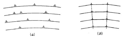
Figure 6-6 Movement of dislocations to produce polygonization (schematic).
