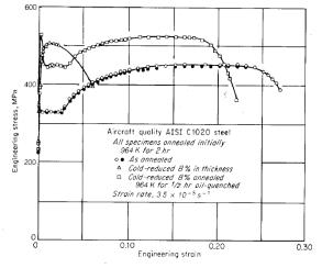
Figure 6-7 Effect of a substructure of low-angle grain boundaries on the stress-strain curve of SAE 1020 steel. (After E. R. Parker and J. Washburn, "Impurities and Imperfections," p. 155, American Society for Metals, Metals Park, Ohio, 1955. By permission of the publishers.)
