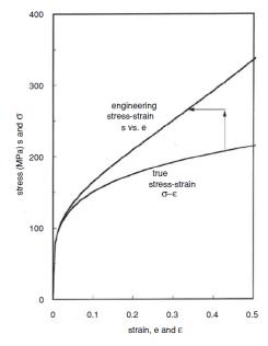
**Figure** Stress–strain relations in compression for a ductile material. Each point  $\sigma$ ,  $\varepsilon$  on the true stress–true strain curve corresponds to a point s, e on the engineering stress–strain curve. The arrows connect these points.
