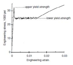
Figure Inhomogeneous yielding of low carbon steel
