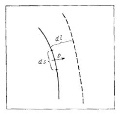
Figure 5-15 Force acting on a dislocation line
