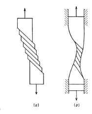
**Figure** 4-20 (a) Tensile deformation of single crystal without constraint; (b) rotation of slip planes due to constraint.
