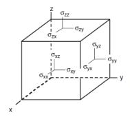
Figure 1.1. The nine components of stress acting on an infinitesimal element. The normal stress components are  $\sigma_{XX}$ ,  $\sigma_{YY}$ , and  $\sigma_{ZZ}$ . The shear stress components are  $\sigma_{YZ}$ ,  $\sigma_{ZX}$ ,  $\sigma_{ZY}$ ,  $\sigma_{ZY}$ ,  $\sigma_{ZY}$ , and  $\sigma_{YX}$ .
