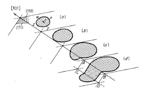
Figure 5-7 Cross slip in a face-centered cubic crystal
