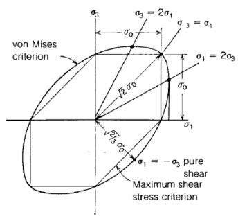
Figure 3-5 Comparison of yield criteria for plane stress.
