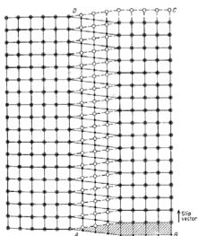
**Figure** Atomic arrangement around the screw dislocation shown in previous Fig.. The plane of the figure is parallel to the slip plane. A BCD is the slipped area, and AD is the screw dislocation. Open circles represent atoms in the atomic plane just above the slip plane, and the solid circles are atoms in the plane just below the slip plane.
