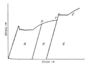
**Figure 6-9** Stress-strain curves for low-carbon steel showing strain aging. **Region A**, original material strained through yield point. **Region B**, immediately retested after reaching point X. **Region C**, reappearance and increase in yield point after aging at 400 K ( $\approx$  130  $^{0}$  C)
