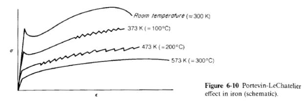
Nitrogen plays a more important role in the strain aging of iron than carbon because it has a higher solubility and diffusion coefficient and produces less complete precipitation during slow cooling. From a practical standpoint it is important to eliminate strain aging in deep-drawing steel because the reap pearance of the yield point can lead to difficulties with surface markings or "stretcher strains" due to the localized heterogeneous deformation.
