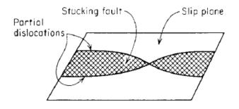
Figure Schematic model of a stacking fault.
