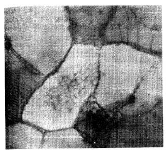
Figure 5-3 Dislocation network in cold-worked aluminum (32,500 X).
