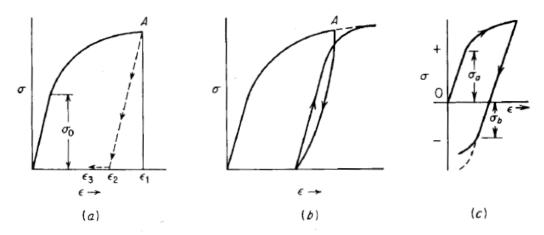
Figure 3-1 Typical true stress-strain curves for a ductile metal.
