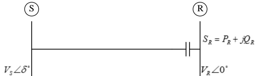
FIG.-3.8 TRANSMISSION LINE WITH SERIES COMPENSATION
