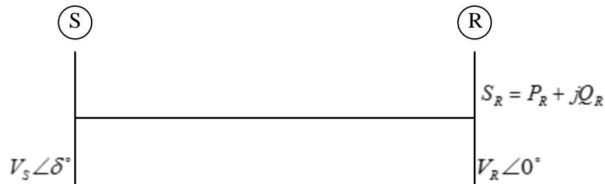
FIG.-3.7 TRANSMISSION LINE POWER FLOW
