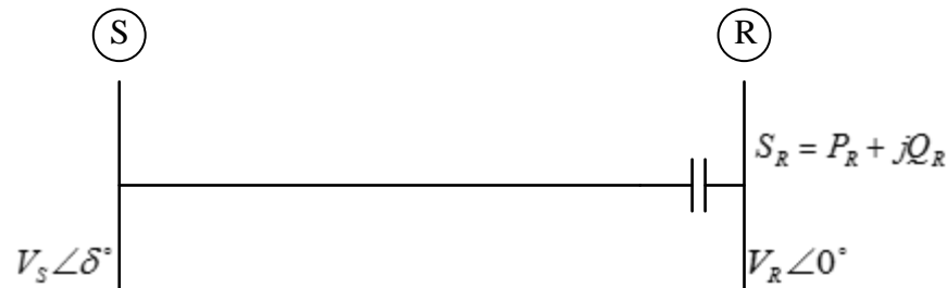
FIG.-11.1 TRANSMISSION LINE WITH SERIES COMPENSATION
