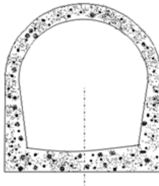
Horse shoe sewer section
