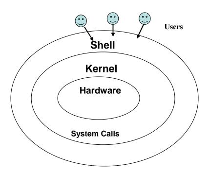
UNIX architecture comprises of two major components viz., the shell and the kernel. The kernel interacts with the machine's hardware and the shell with the user.
